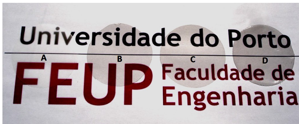
Figure 10 – Images of PLA and PLA + GO films. A - PLA, B - PLA + 0.2 wt. %, C - PLA + 0.4 wt. %, D - PLA + 0.6 wt. %.
