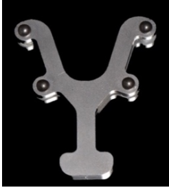
Figure 10. Metallic reference aid with four steel spheres. Font: Schmidt et al. 2020 (29)
