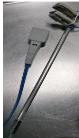
Figure 2- Custom-made Sensor Holder
