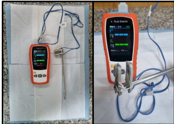
Figure 2: custom PO probe. Its form permitted parallel positioning of the emitter and the sensor, although its form did not always accommodate tooth's structure
