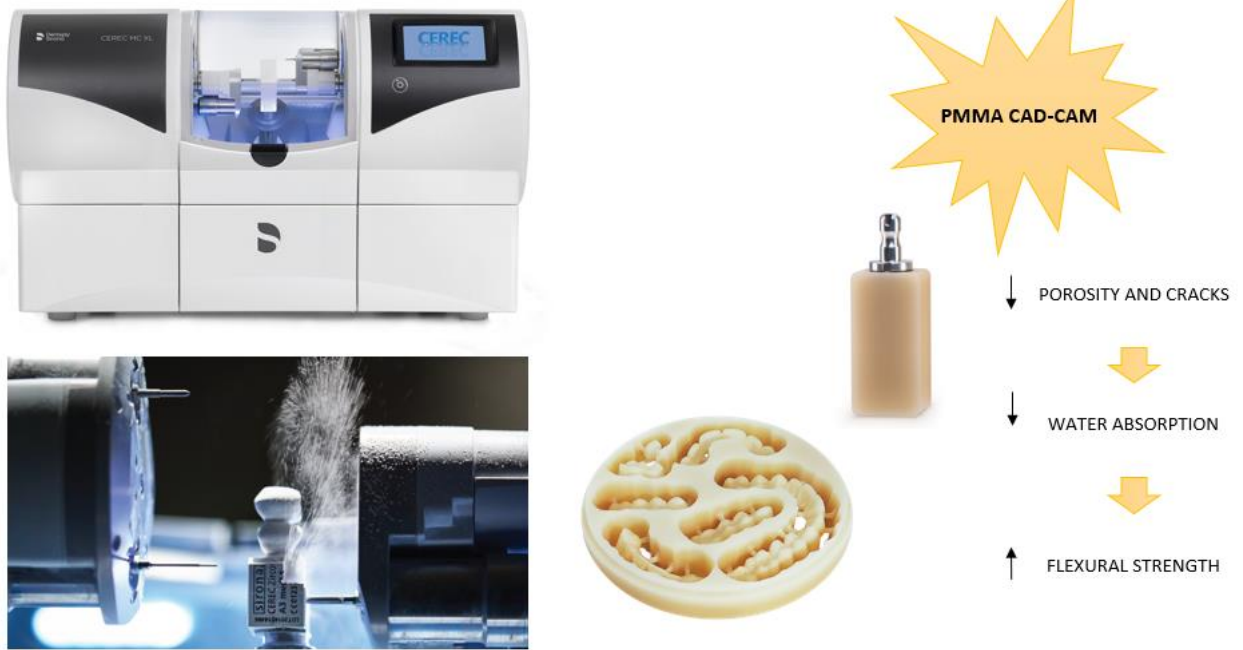
Figure 2. Schematic representation of PMMA material manufactured by CAD-CAM.
