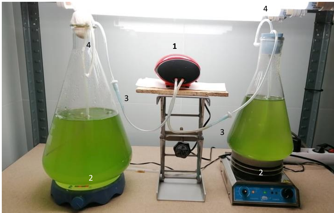
Figure 7 – Microalgae culture: Erlenmeyer containing the microalgae culture (1 - air pump system; 2 - magnetic agitation; 3 - filtered air supply with a 0.22 \mu\text{m} filter; 4 - tube for air flow out).
