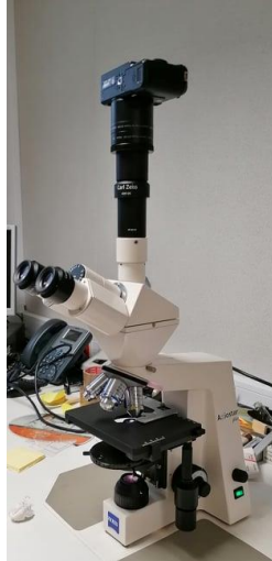
Figure 11 - Optical microscope coupled to a digital camera for photograph and video recording.
