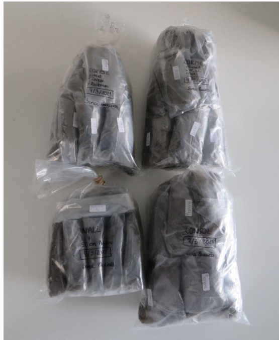
Figure 15: Plastic bags with grave inner soil samples packed within other different plastic bags (CORPSE - two bags with the samples collected under the corpse; WALL + 100 centimetre Auger - one bag with the samples collected from the grave walls and from the right corner of the grave; CONTROL - one bag with the samples collected from locations with no human decomposition activity).
