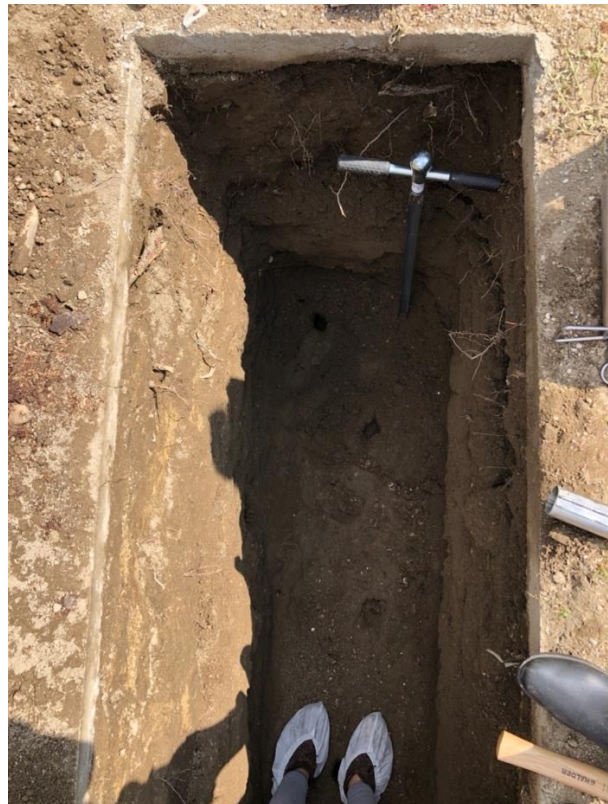
Figure 12: 100 centimetre sampling Auger (04010330V, Eijkelkamp Soil & Water) sampling soil's profile at the right corner of the grave (head side of the corpse).
