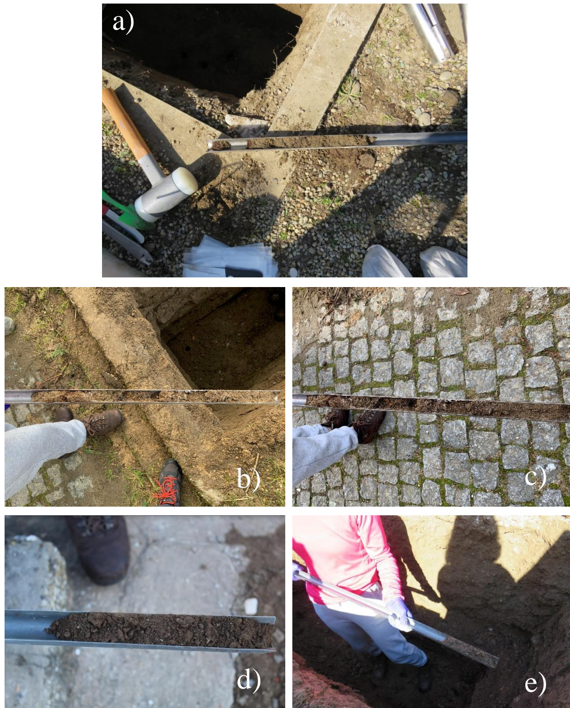
Figure 16: Soil's profiles, collected using the 100 centimetre auger, from exhumations in Monte D'Arcos Cemetery (a-c) and from exhumations in Castelo de Mértola Cemetery (d and e).
