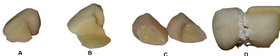
Figure 60 - Details of fractured RBBs and the most frequent mode of failure by material type. (A) ENA, adhesive on the interproximal surface and cohesive in the retainer; (B) Y-ZPT, adhesive with RBB integrity; (C) SUP, cohesive in Frasco tooth and retainer; (D) ABS, adhesive on the interproximal, cohesive with plastic deformation in RBB
