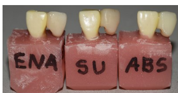
Figure 55 - Example of ENA, SUP, and ABS RBBs ready for the SBS test.
