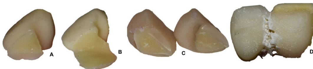
Fig. 6 Details of fractured RBBs and more frequent failure modes by material type. (A) ENA, adhesive interproximal and cohesive in retainer; (B) Y-ZPT, adhesive, with RBB integrity; (C) SUP, cohesive in Frasco tooth and retainer; (D) ABS, adhesive in interproximal, cohesive with plastic deformation in RBB (no RBBs' tooth loss occurred)
