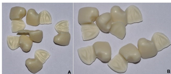
Figure 53 - Adhesion surface of RBB Y-ZPT (A) before and (B) after surface treatment with Al 2 O 3 sandblasting with loss of the slight glossy surface generated by milling
