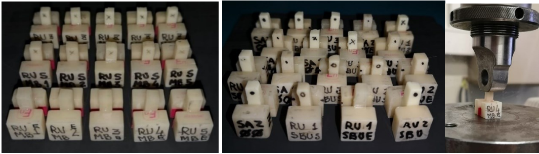
Figure 36 - Specimens prepared for the shear bond test, according to the adhesive cement, surface treatment of the base and bar and coupling agent used, together with a detail of the loading procedure
