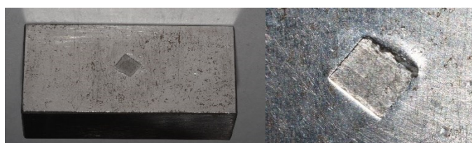
Figure 41 - Pressure mark on the tempered steel support made by the Y-ZPT cube during the compression strain test
