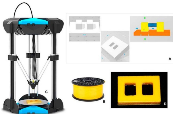
Figure 8. Steps of the polylactic acid (PLA) base design and fabrication. (A) design steps; (B) PLA coil; (C) PLA base in the printing process; (D) PLA base just printed.
