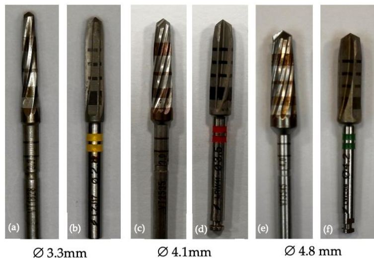
Figure 1. The configuration of the final drill used for each group (SD and OD). (a) VT1828; (b) Ø 2.8 BLT Drill; (c) VT2535; (d) Ø 3.5 BLT Drill; (e) VT3545; (f) Ø 4.2 BLT Drill.
