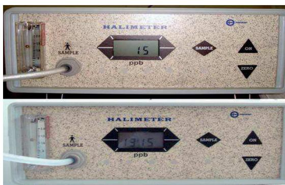
Figura 8-Monitor portátil de sulfetos :HALIMETER® (Interscan Co. Chatsworth,CA).(27)
