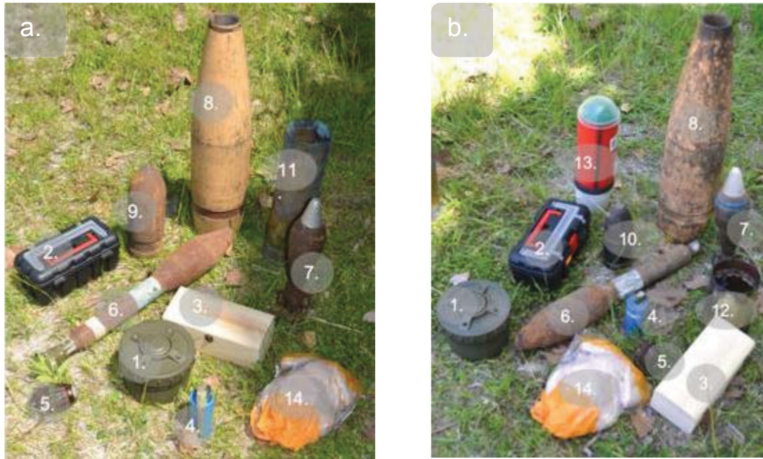
Figure 10. Targets buried in the sandy soil study site (a) and in the clayey soil study site (b): (1) antipersonnel mines; (2) improvised explosive devices in a plastic box; (3) improvised explosive devices in a wooden box; (4) Instruction hand grenades Mod/962; (5) MILLS hand grenades; (6) rockets; (7) 81 mm mortar grenades; (8) 155 mm artillery projectiles; (9) 80 mm artillery projectile; (10) 60 mm artillery projectile; (11) 101 mm artillery case; (12) 105 mm blank M365 cartridge case; (13) FIREND; (14) chicken.
