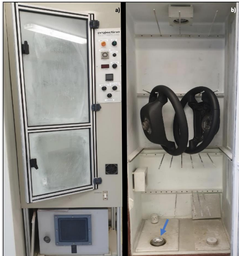
Figure 15 - Cyanoacrylate Projectina® fuming chamber: a) external view and b) internal view (blue arrow=aluminium container).
