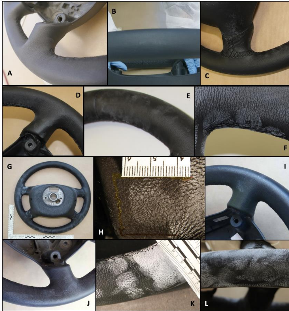
Figure 30 - Driven steering wheels developed with cyanoacrylate fuming (A-L=volunteers codified according to the sampling sequence).
